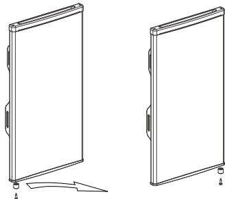
5) Install the door on the lower hinge assembly, and then install the upper hinge, hinge cover, pins and hole cap in sequence.
