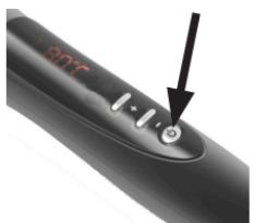
4. Switch on the curl styler by pressing the ON/OFF button [6]. The heat-up phase is indicated by the temperature display flashing. When the temperature display is continuously lit, the curl styler has reached the set temperature setting and can be used.
