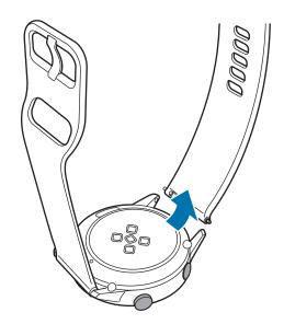
3 Insert one end of the spring bar's new band into the Galaxy Watch Active's lug.
