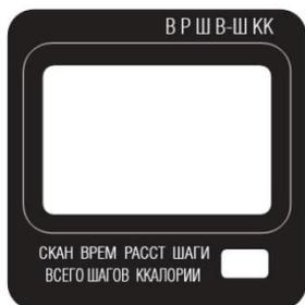
Press the red button to turn on the display. You can select the display of the desired indicator by repeatedly pressing the red button until the pointer (triangular arrow at the top of the display) moves to the desired division (В, Р, Ш, В-Ш или ККАЛЛ). See the top right corner of the display for a list of functions.
