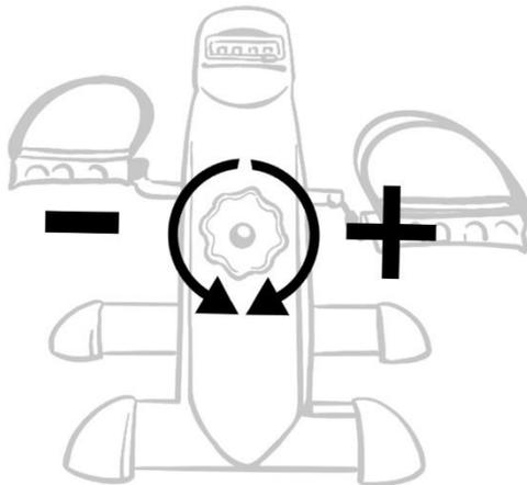
To increase the load, turn the knob clockwise and counterclockwise to decrease the load, respectively.
