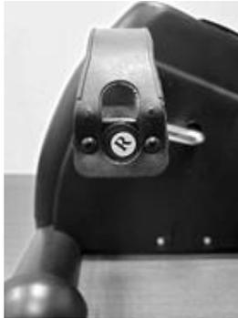
The screws are fixed at the same level as shown in the picture above. Lock the screws on the lower level if you want to make the leg restraint wider and on the upper level if you need to narrow it down.
