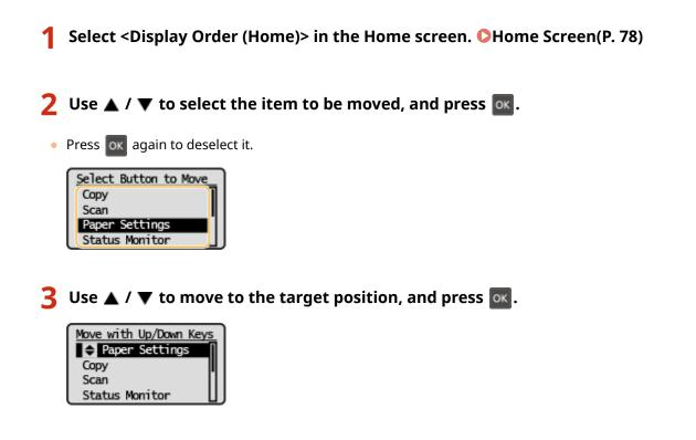
**4** When the buttons are rearranged in the way you want, press the Back key.
