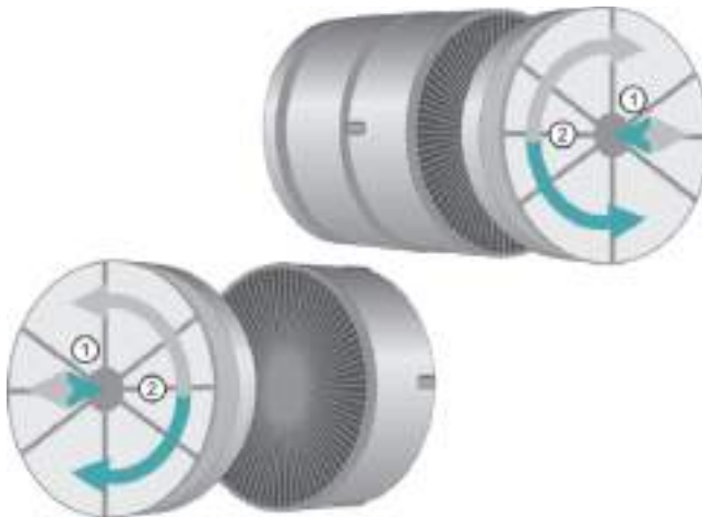
Pic. 14 Carbon filter installation
