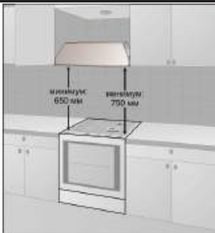
Fig.6 Minimum distance from gas and electric stove
