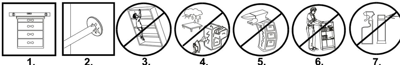
1. Furniture units must be placed on a level surface and levelled.
