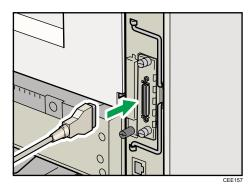
3. Connect the other end of the interface cable to your computer, and then secure the cable.
