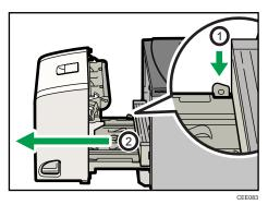
5. Lift the lock levers of the fusing unit as shown in the illustration.
