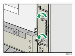
4. Fully insert the Wireless LAN interface board.
