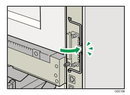
13. Fasten the controller board to the printer with the two screws.
