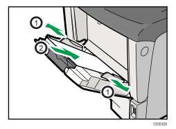
3. Adjust the paper guide both sides to fit the paper width.
