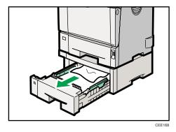
If paper jams occur in multiple trays, a message indicating multiple trays such as "(Y2)" appears. Open all the trays indicated on the control panel, and then remove the jammed paper.
