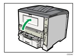
12. If the optional duplex unit was removed, re-install it in the printer by pushing it along the rails on the inside of the printer.
