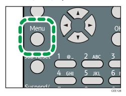
2. Press the [▼] or [▲] key to select [Paper Input], and then press the [OK] key.
