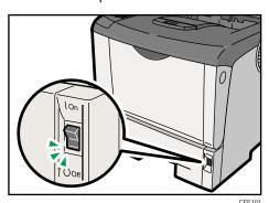
2. Plug in the power cable, and securely insert the plug of the power cord into the wall socket.
