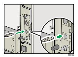
2. Connect the opposite end's flat connector to the desired device such as your computer's USB interface, or a USB hub.
