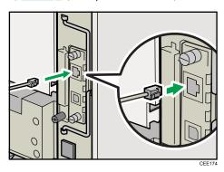
3. Connect the other end of the cable to the network, for example using a hub.
