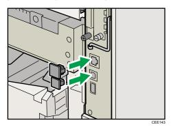
4. Remove the two screws and remove the cover of the slot in which the Gigabit Ethernet board is installed.
