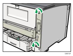
The removed screws are required to fasten the controller board.
