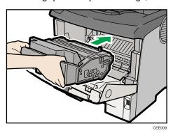
8. Push down the print cartridge to secure it in the appropriate position.
