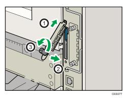
If ELP-NX card is inserted in the printer, the installation automatically starts when the printer is turned on. After the installation is completed, restart the printer.
