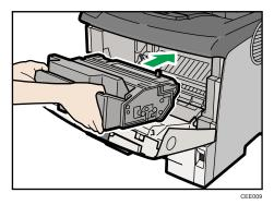
10. Push down the print cartridge to secure it in the appropriate position.
