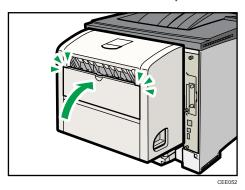
4. Lift the lever (1), open the cover of the duplex unit (2).
