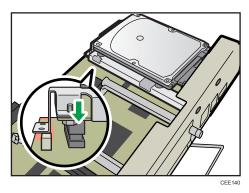
9. Tighten the two screws by turning them clockwise with a coin, and then secure the hard disk board by tightening the third screw from the under side of the controller board.
