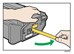
8. Pull out the tape from inside the unit horizontally while holding the cartridge with one hand as shown in the illustration.
