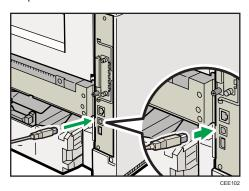
Connecting the USB cable to the Gigabit Ethernet board USB port
