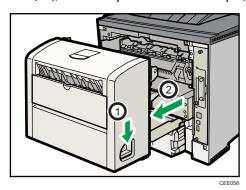
4. Push the under board levers ( $\bigcirc$ ), and then pull the duplex unit out of the printer ( $\bigcirc$ ).
