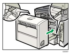
13. Securely push the duplex unit into the printer.
