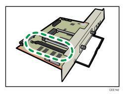
6. To install the recommended memory, align the notch of the recommended memory with the protruding part of the vacant slot, and then carefully insert the module at an angle.
