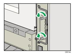
5. Fully insert the Gigabit Ethernet board.
