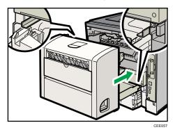
11. Push the duplex unit securely into the printer.
