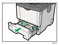
4. Lift the front side of the tray, and then pull it out of the printer.
