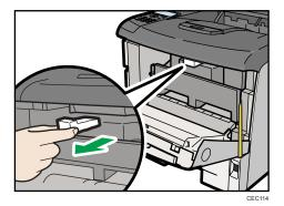
6. Lift the front side of the print cartridge, and then pull it out of the printer.
