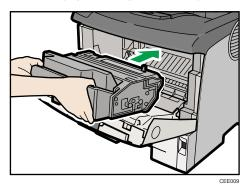
7. Push down the print cartridge to secure it in the appropriate position.
