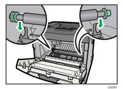
7. Push down the lock levers on both ends of the printer as shown in the illustration, until they click into place.
