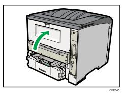
6. If the optional duplex unit was removed, re-install it in the printer by pushing it along the rails on the inside of the printer.
