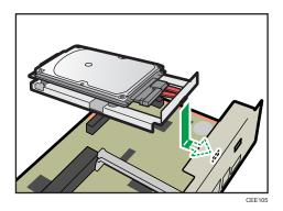
8. Fit the hard disk on the connector of the controller board carefully until it stops.
