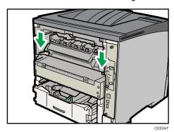
10. Position the rear cover horizontally and align it with the grooves in the printer's interior.
