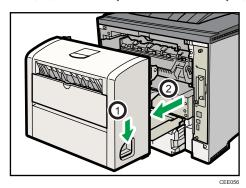
4. Push the under board levers (1) and then pull the duplex unit out of the printer (2).
