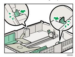
4. Pinch the clip on the side paper guide and slide it to match the standard size.
