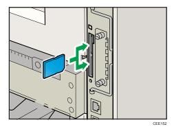
If you insert only one SD card, use the upper slot. If you insert two SD cards simultaneously, use both slots. If you insert the optional VM card, use only the lower slot.
