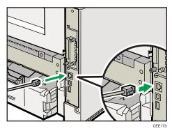
3. Connect the other end of the cable to the network, such as a hub.
