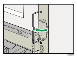
5. Pull the handle, and then slide the controller board out.
