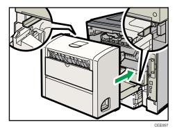
13. Securely push the duplex unit into the printer.
