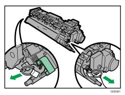
8. Push the new fusing unit into the printer.
