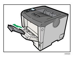
2. Slide the paper guide both sides outward, and then load paper print side up, until it stops.
