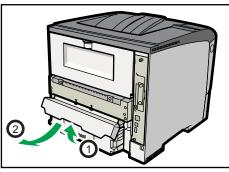
10. Hold the tray with both hands, slide it along the rails of the printer body, and then push it straight in.
