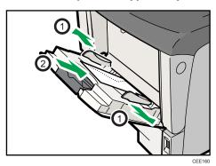
When loading envelopes, be sure to load envelopes in the tray with their closed flaps facing the left side of the tray.
