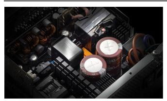
XPG CYBERCORE PLATINUM Series utilizes all-Japanese high quality 105 °C - grade capacitors to ensure power delivery is stable, consistent and efficient.
