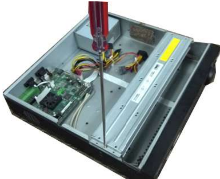
Figure 3-37 Open the top cover
