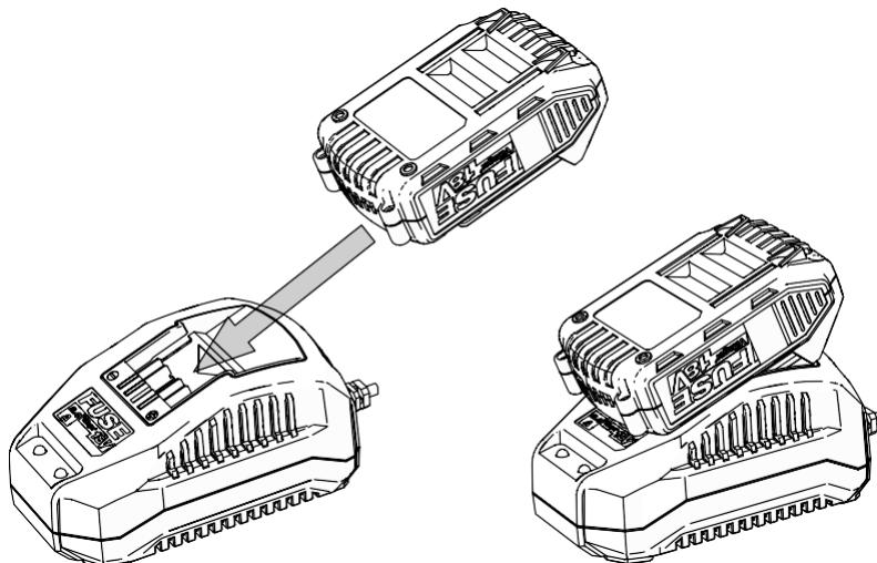
3. When the battery is fully charged, the red LED goes off and only the green LED stays on.
