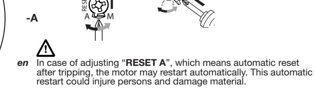
**en** In case of adjusting "RESET A", which means automatic reset after tripping, the motor may restart automatically. This automatic restart could injure persons and damage material.
