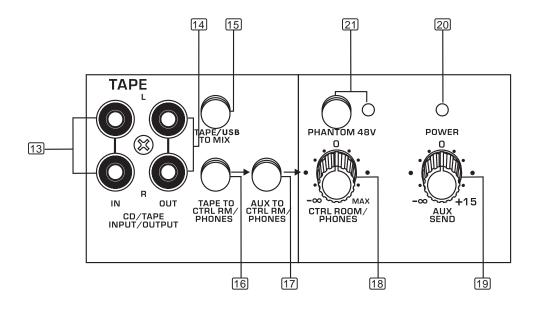
15- TAPE/USB V2 TO MIX Switch(USB V2 For MX.6USB V2, MX.10USB V2, MX.12USB V2) Connect a CD or Tape Deck to the CD/TAPE inputs, and push down this switch to add the CD/TAPE signal or USB V2 Audio interface signal (MX.6USB V2, MX.10USB V2, MX.12USB V2) to the main mix. The volume level is controlled by MAIN MIX control.
