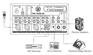
In this case up to three Musicians (Vocalist, Guitar Player & Keyboard Player) can hookup to the TPS 16AM.UB and an additional Drum Machine can also be connected to the Stereo Channel. One or two external passive speakers can be connected (the internal speakers will not be affected) as well as a powered stage Monitor.
