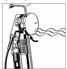
Backflow situation: If a negative pressure situation should occur when the bathtub is filled, there is a possibility that bath water may flow back into the drinking water system.
