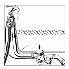
The drain / overflow are controlled via rotatable rosette on the overflow. Proceed as follows to open or close the drain:
