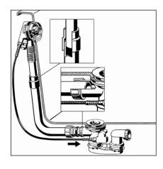
Hold the pipe of the overflow unit parallel to the overflow pipe and mark the positions where the drain and the overflow should be connected.
