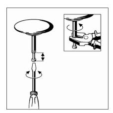
Turn rotatable rosette to check function and alignment.
