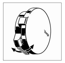
Push the flow control backwards or forwards with your finger. The water flows closer or further away from the side of the bathtub depending on the direction set.
