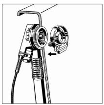
Fit inlet flange into the overflow unit.
