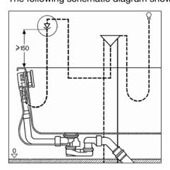
Fig. 2: Mounting scheme with pipe interrupter
