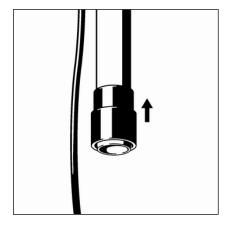
Push the rubber sleeve onto the overflow unit pipe until the lower edge is flush with the edge of the overflow pipe.
