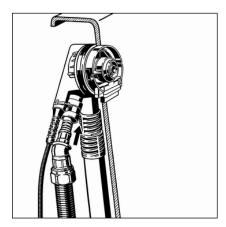
Insert the inlet adapter into the overflow unit.
