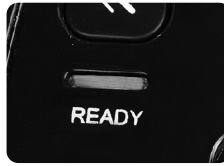
(Fig.2) The machine is ready to use when you hear the beep sound and the READY LIGHT turns to green and stays steady.
