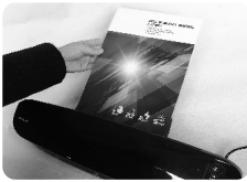
(Fig.4) The laminating process is finished when the whole document comes out from the other end of the machine.
