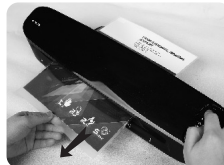
(Fig.5) If the pouch gets jammed inside, you will hear the beep sound. Press the REVERSE BUTTON and hold it until the pouch is removed.
