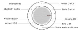
The CP900 can connect to PC via USB cable or Bluetooth, and to smartphone via Bluetooth. After connected, you can control the calls on the CP900.
