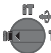
Position for drilling without impact in wood, metal, ceramic and plastic as well as for screwdriving
