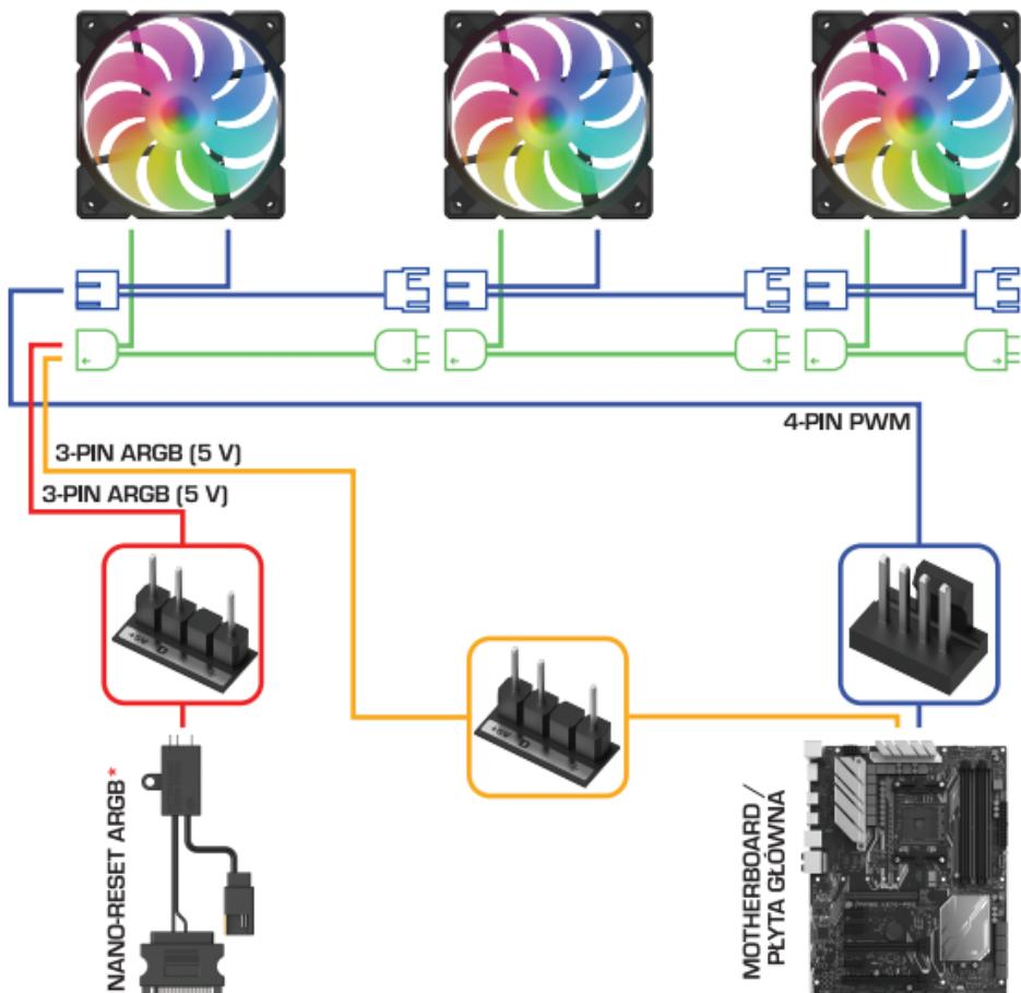
A EN: Choose A if you have a motherboard with 3-pin ARGB socket and want to control the ARGB lighting using the software from your motherboard manufacturer. If you chose B (control via motherboard), connect the individual elements according to the yellow lines only.
