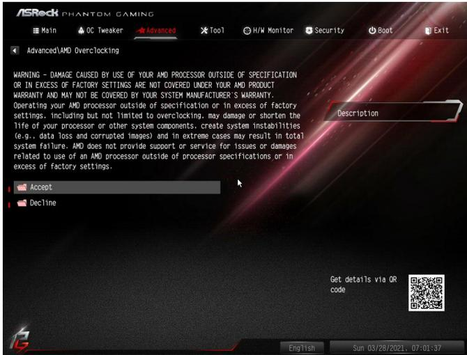
The AMD Overclocking menu accesses options for configuring CPU frequency and voltage.
