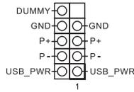
There is one header on this motherboard. This USB 2.0 header can support two ports.
