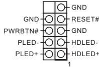
Connect the power button, reset button and system status indicator on the chassis to this header according to the pin assignments below. Note the positive and negative pins before connecting the cables.
