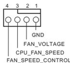
This motherboard provides a 4-Pin water cooling CPU fan connector. If you plan to connect a 3-Pin CPU water cooler fan, please connect it to Pin 1-3.
