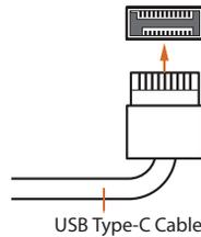
There is one Front Panel Type C USB 3.2 Gen2 Header on this motherboard. This header is used for connecting a USB 3.2 Gen2 module for additional USB 3.2 Gen2 ports.
