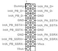
There is one header on this motherboard. This USB 3.2 Gen1 header can support two ports.
