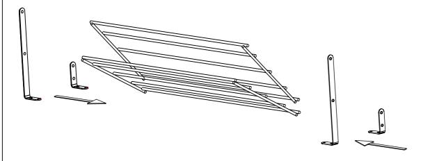
2- Fix long and small L-shaped part to cabinet doors with chipboard screw.
