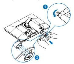
3. Remove the screws from hinge cover.
