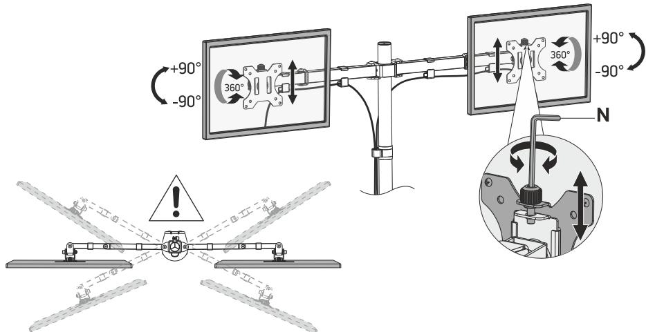
**IMPORTANT:** DO NOT overtighten mounting screws, it can damage the mount and your equipment.
