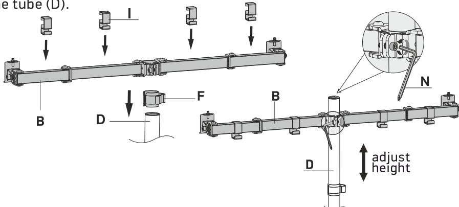
Install mounting arm (B) on the tube (D). Set desirable height of the arm and tighten screws by using key (N).
