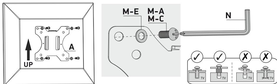
Other screws (M-B), (M-D), washers (M-E) and spacers (M-F) can be used as required. You may use the key (N). Make sure VESA panels are securely fixed. Look carefully at the picture below:
