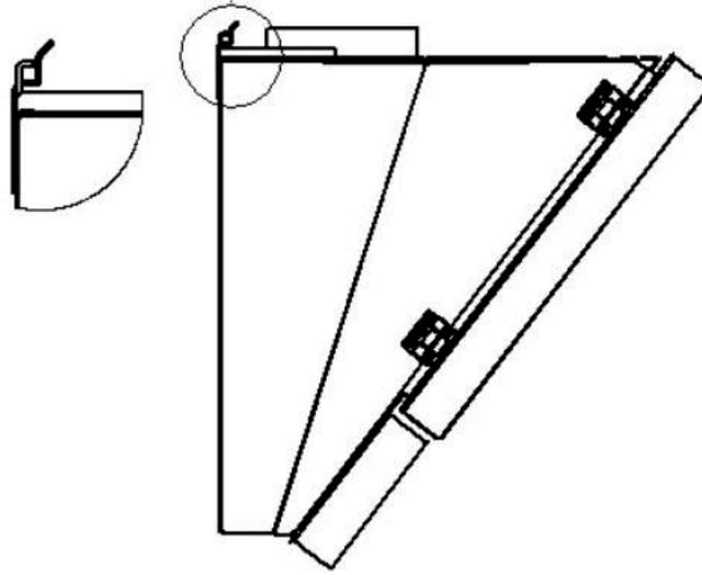
**Aluminum pipe fiGng:** One end of the aluminum pipe is the plastic bacquet on the product; And the other end to the kitchen sink. Make sure that these two connectors are tight enough that they will not come out of place when the hood is operating at the highest speed. The diameter of plastic bacan on the product is 150 mm. If aluminum pipe with a diameter of 120 mm is to be used, it is necessary to install a plastic reducer from the packaging.
