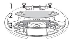
3. Replace the nozzle using a 7 mm spanner according to the gas to be used.
