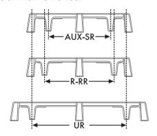
The continuous contact between the pan supports and the flame can cause modifications to the enamel over time in those parts exposed to heat. This is a completely natural phenomenon which has no effect on the operation of this component.
