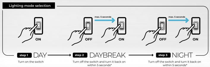
\*If the switch is turned on again after more than 5 seconds, the light will cycle back to the Day mode
