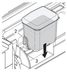
4. Push the water reservoir downwards so that the water can flow into the ice tray.
