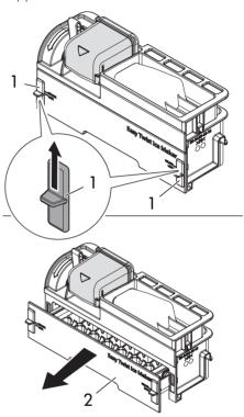
2. When replacing the ice tray and its holder, secure the hooks to prevent it from moving.
