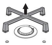
2. Remove the flame-spreader crowns and relative burner caps.
