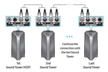
Set up Group Play by connecting all the systems using audio cables (not supplied). Use the **AUX** or **Source**) button to change the source to **AUX2** for every Sound Tower system except the 1st (or HOST) Sound Tower system.
