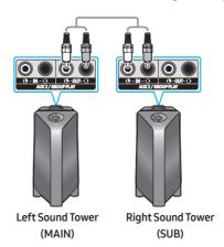
1. Refer to "Using a Smartphone and Stereo Group mode" to connect the two Sound Towers in a Stereo Group.
