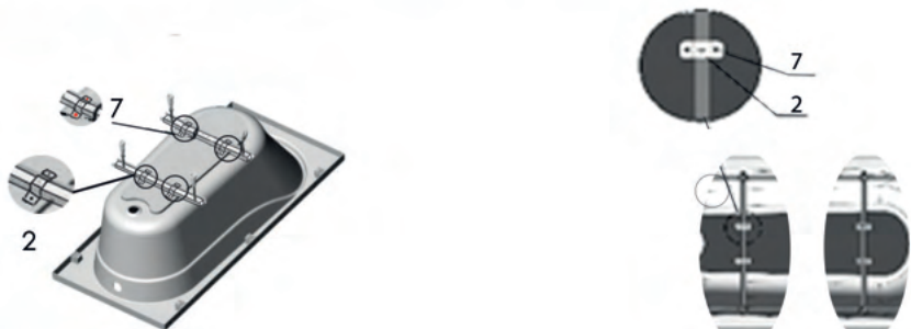
Pic.5 bath legs fixation
