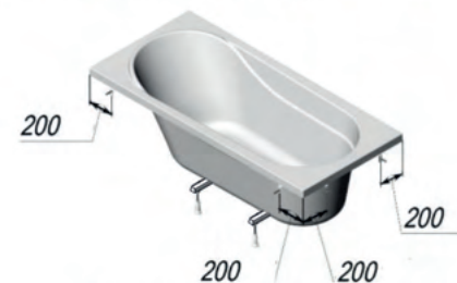
Pic.6 fixation of the bathtub to the wall
