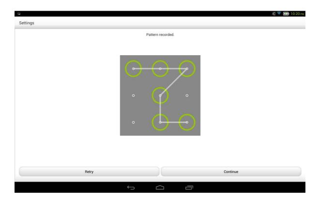
After you have set and activated the pattern unlock function, the unlock keypad will be displayed whenever the display is to be unlocked. Use your finger to trace your preset pattern on the keypad. After the preset pattern has been correctly entered, the screen will be unlocked.
