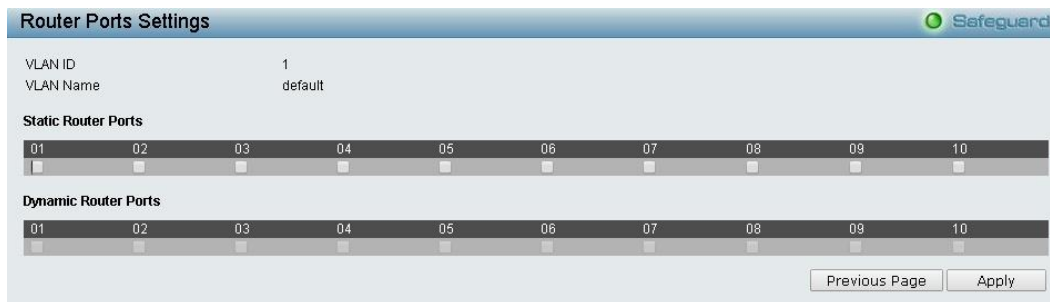
Figure 4.60 – Configuration > MLD Snooping > MLD Snooping-Router Port Settings
