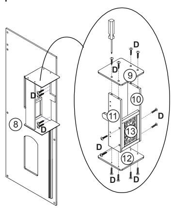
Wait to assemble part 10 until after elevator is assembled to the track pieces.
