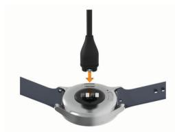
**3** Plug the USB cable into a power source to turn on the device (*Charging the Device*, page 10).
