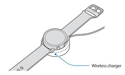
**3** After fully charging, disconnect the Galaxy Watch Active2 from the wireless charger. First, disconnect the wireless charger from the charger and then unplug the charger from the electric socket.
