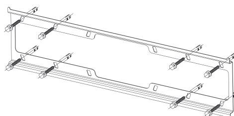
*Using A plate as a template and the level of the sets, mark the place of the installation according to the mounting holes in the plate A; holes should be placed horizontally Using a punch, drill the holes in the wall with a diameter of 10 mm and a depth of not less than 60 mm. Put the dowels C in the holes. Fasten the plate A to the wall using the screws and the washers from the set C.*
