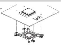
Apply thermal grease just enough to thinly cover the CPU surface, then fasten the Bolts to isntall the cooler.
