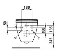
Connection with Laufen installation system LIS CW2
