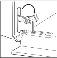
Close the oven door halfway to the first opening position. Then lift and pull forward and remove the door from its seat.
