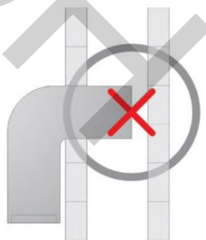
Fig.7 b. Connections of plastic corrugated tube
