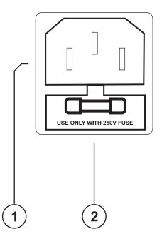
**1.) AC Power Cord Receptacle -** AC power cord can be removed for easy storage and replacement if damaged. Insert the AC cord (provided) firmly into the AC receptacle. **NOTE:** Replace the AC power cord if protective jacket is damaged or ground pin is damaged or removed.
