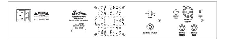
**External Speaker:** This is a two-conductor, <sup>1</sup>/<sub>4</sub>-inch external speaker jack. (*Note:* This jack is wired in series with the amp's internal speaker. Therefore, the internal speaker still functions when an external speaker cabinet is added. For this reason, there is no minimum external speaker impedance load.)
