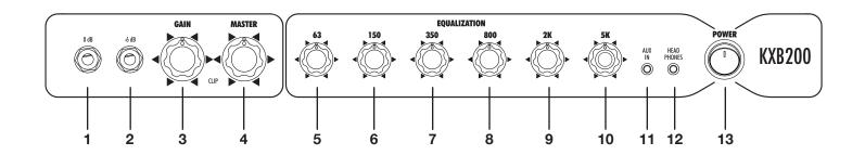
**1. 0 dB Input:** <sup>1</sup>/<sub>4</sub>-inch input that is intended for bass guitars with standard, passive electronics.
