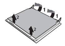
3. Some models have an intermediate glass pane. Remove the intermediate glass pane by lifting it upwards.
