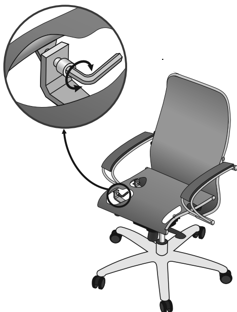
Dual-zone seat stiffness adjustment
