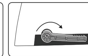
3. Ensure the comb-opening mechanism is closed.
