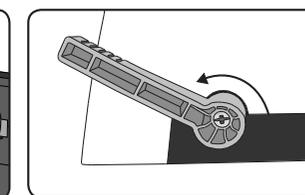
3. Open the binding comb by turning the comb lever. Take care not to open the comb too far.
