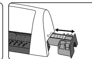
2. Lift the punch handle. Check the waste tray is empty and correctly fitted.
