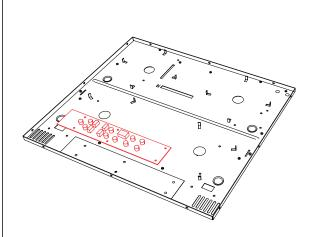
Step 7: remove the display board
