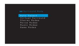
**Auto Select:** For digital programs, such as a movie recorded with a Dolby Digital or DTS soundtrack, the AVR will automatically use the soundtrack's native surround format. For two-channel analog and PCM programs, the AVR uses the Logic 7 Movie or 2CH Stereo mode, depending on the source.
