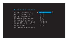
**Panel Timeout:** This setting allows you to set the AVR's front-panel display to automatically turn off after remaining on for a predertimined time (3 - 10 seconds) each time you use a control. Set this to "Off" to have the display remain on continually.
