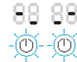
Water treatment: The AM10 is treating the water. This takes 3 minutes. When the animation stops, the AM10 will start to humidify.
