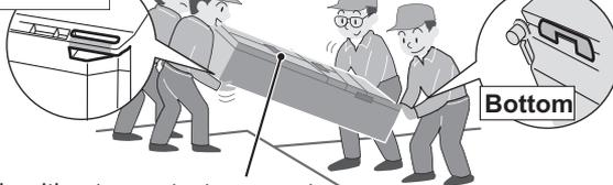
Fix with a tape, etc. to prevent the doors from opening.
