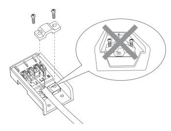
5. Assemble the cable clamp, be aware that the ellipse hole on cable clamp must match the ellipse hole on.
