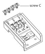
4. Remove the 4 screws C in the terminal box and insert the power cord at the connection.
