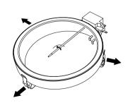
Step 3: open the bracket and remove the heating element
