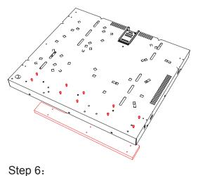
to remove the display board fixing box, reverse the base and remove the screws
