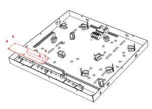
Step 5: remove the power board
