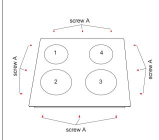
Step1: remove the screw A around the base cover
